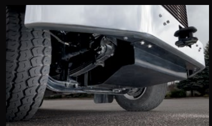
One-piece skid plate for under-chassis protection.
