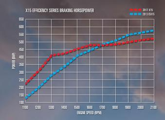
X 15 EFFICIENCY SERIES Braking Horsepower.
