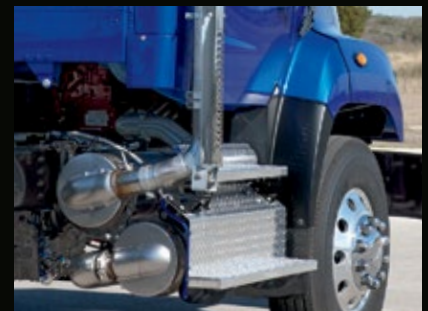
Exhaust aftertreatment system packaged under cab for ease of body upfit.
