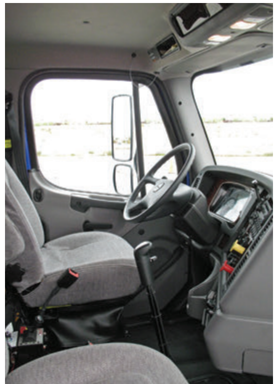
Cab is wide enough for three people, but this one's set up for two. Controls for the dump body are between the seats.
