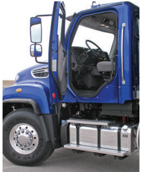
Aluminum cab from the M2 series was originally designed for vocational use, so is strong enough for the SD series, Freightliner says.
