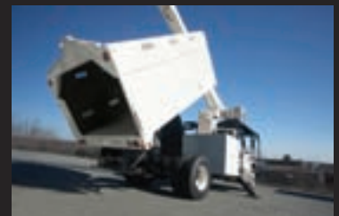
Chip boxes are available with dump capability.
