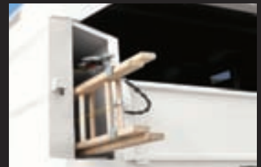
Rear storage compartments safely store ladders and other long tools.
