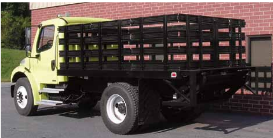
Stake Body Installations
