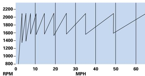
Based on engine operating at 2100 RPM and top speed of 65 MPH.
