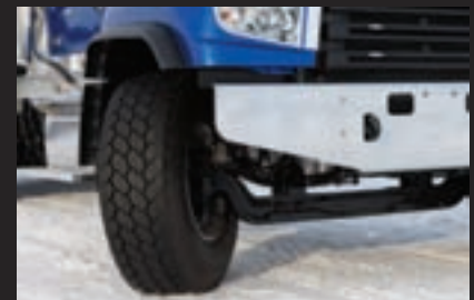
Up to 45 degree wheel cut depending on wheel equipment.
