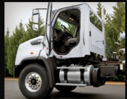
65 degree door opening for ease of entry/exit.
