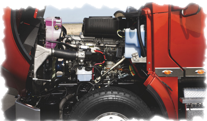
The Coronado® 122SD radiator and fan are mounted to the engine instead of the frame rails to isolate the radiator from chassis shock loads which reduce vibration.
