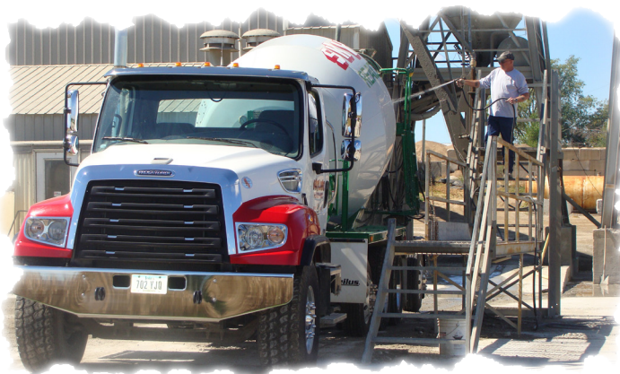
This hard-working Freightliner 114SD was fitted with a 10.5 cubic yard McNeilus Bridgemaster® Transit Mixer for a 2011 trade show.
