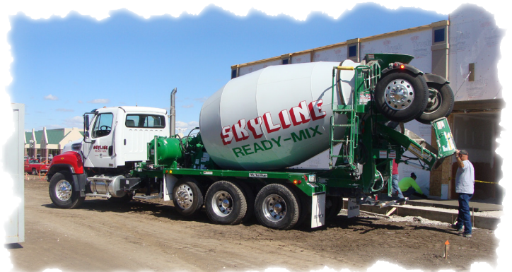
Skyline Ready-Mix uses this Freightliner® 114SD for hauling ready-mix concrete for everything from paving roads to building houses.
