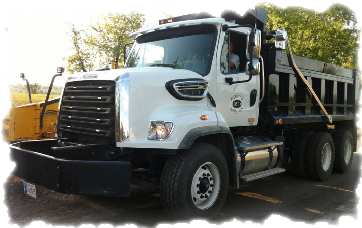
Wagoner County has upfit the new 108SD as a spreader/snowplow that is used after winter as a dump truck in road construction work. It can be converted in a day, so no matter what the conditions, this truck can keep on working.
