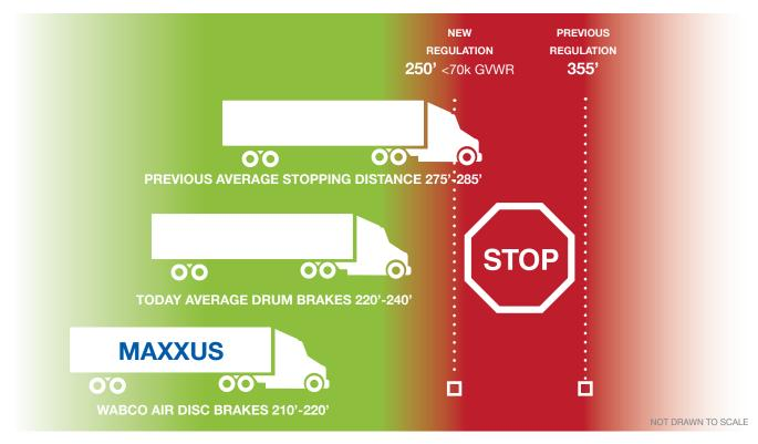
WABCO MAXXUS provides increased braking capabilities to exceed new federal stopping distance requirements.
