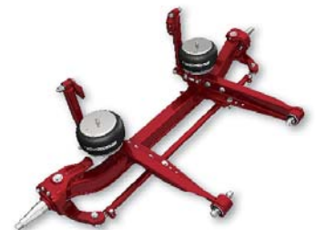
STEERTEK NXT with leading arm suspension
