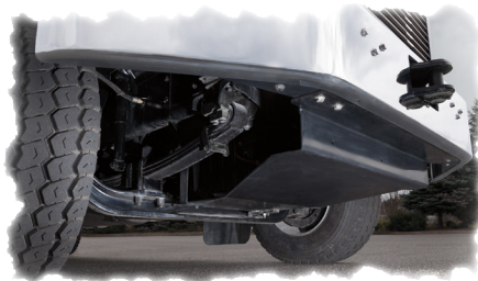
A Freightliner Coronado 122SD logging truck. Without a skid plate, deep mud, rocks and stumps can damage the undercarriage of a truck.
